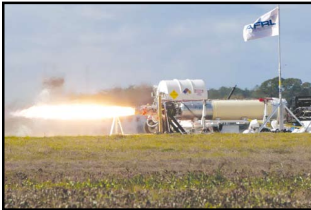
A X-60A hot fire test is conducted at Cecil Spaceport in Jacksonville, Fla., Jan. 14, 2020. The X-60A, developed through an Air Force Research Laboratory Small Business Innovation Research contract, is an air-launched rocket designed for hypersonic flight research. U.S. Air Force photo courtesy of Air Force Research Laboratory
