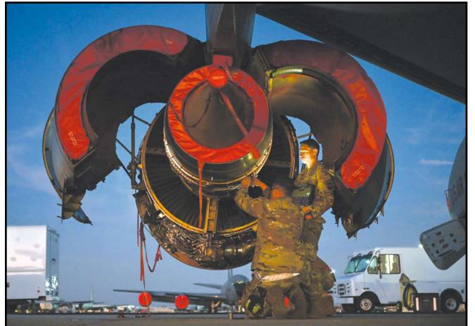
TAKING A LOOK UNDER THE HOOD Aerospace propulsion Airmen assigned to the 6th Maintenance Squadron inspect the engine of a KC-135 Stratotanker at MacDill Air Force Base, Fla., earlier this month. Aerospace propulsion specialists are responsible for the maintenance, repair and testing of aircraft engines, turbines and other propulsion systems. U.S. Air Force photo by Senior Airman Derrick Bole
